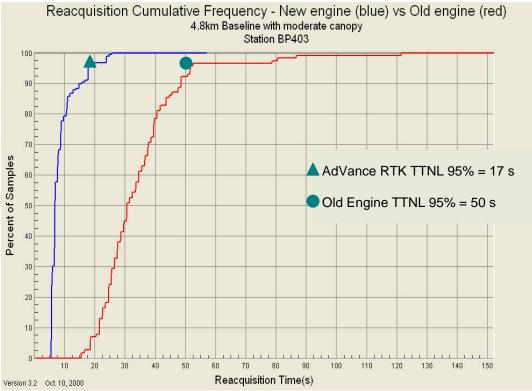
Figure 5: Reacquistion Time Under Moderate Canopy
