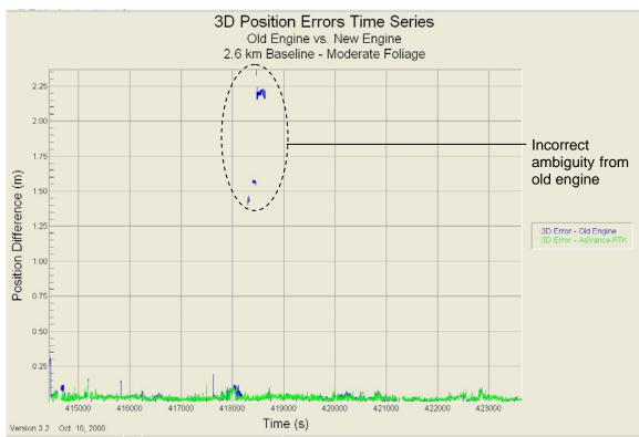
Figure 8: Old Engine vs AdVance RTK Horizonatal Position Error
