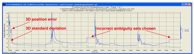
Figure 12: Old Engine's Position Difference in Foliage
