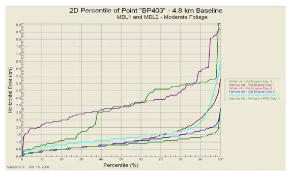
Figure 11: Both Engine's Position Error at 4.8 km Baseline
